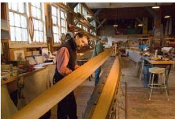
Steve Chapin carefully removes the first of two steam bent cedar planks from the original Pocock form.
